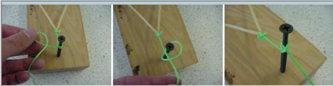
Figure 5. Tying a single hitch knot Copyright © Photograph taken by Jeff White, University of Colorado at Boulder, 2003.
